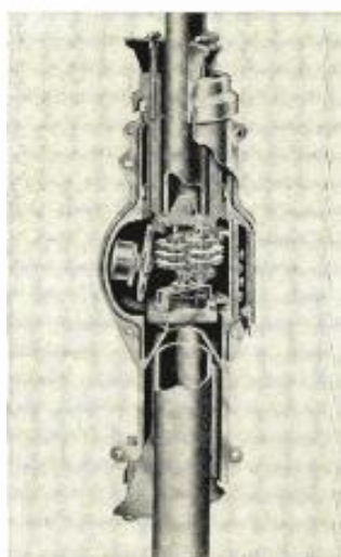
Fig. 2. Cutaway view of the Vee-D-X antenna rotator showing how the drive mechanism is positioned to allow the antenna mast to be in line with the support mast.
