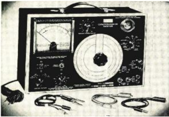
The Pyramid model CRA-1 capacitor and resistor analyzer.
