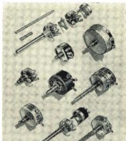
Fig. 12. Various types and sizes of potentiometers are shown here, both carbon and wirewound. These are from Mallory.
